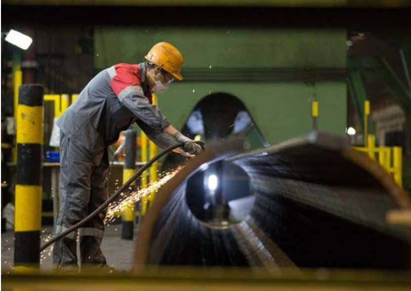
A worker grinds the edges of a rolled steel pipe for use in the South Stream gas pipeline at the Vyksa Steel Works, operated by United Metallurgical, in Vyksa, Russia, on Tuesday. Russian equities trading in New York fell for a third day, the longest slide in a month. (Photo: Andrey Rudakov, Bloomberg)
