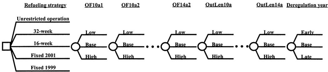
Figure 5: This schematic decision tree with over 200 million endpoints shows the scenarios to be evaluated for each of the New York Power Authority’s refueling strategies for the Indian Point 3 Nuclear Power Plant. Uncertainties include operating factors (OF10a1, OF10a2, . . . , OF14a2), outage lengths (OutLen10a, . . . , OutLen14a), and deregulation year.
