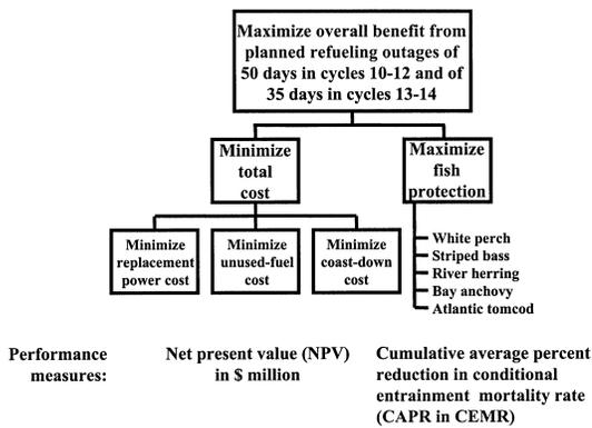
Figure 2: The objectives hierarchy shows the objectives and performance measures we used to compare strategies for scheduling refueling outages at the New York Power Authority's Indian Point 3 Nuclear Power Plant.
