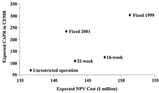
Figure 8: The relative rank of five refueling strategies for the New York Power Authority’s Indian Point 3 Nuclear Power Plant is based on both expected net present value (NPV) of cost and fish protection, expressed as the expected cumulative average percent reduction in the conditional entrainment mortality rate (CAPR in CEMR). Both lower values of NPV cost and higher values of CAPR in CEMR are better.
