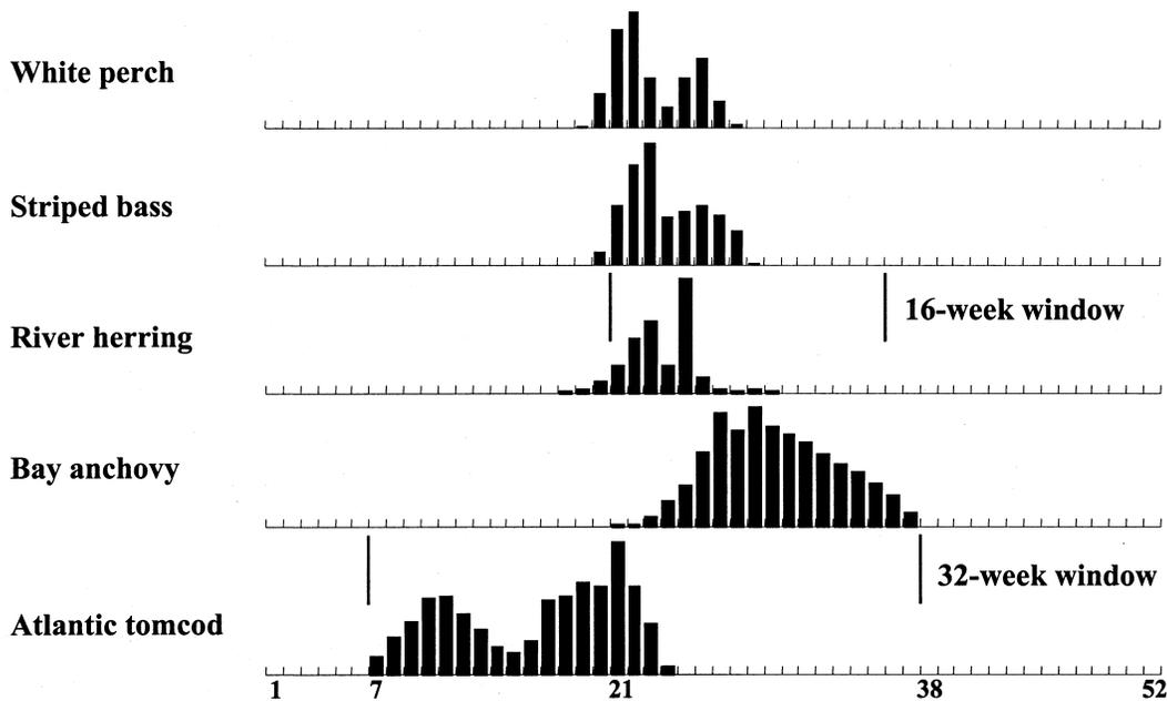
Figure 3: This figure shows the relative contribution by week to the maximum, annual conditional entrainment mortality rate (CEMR) for five taxa of fish at the New York Power Authority’s Indian Point 3 Nuclear Power Plant (IP3). If IP3 did not operate during the 32-week window, the CEMR for each taxon would be reduced to zero.
